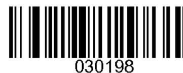
Tip: when scanning Reset para. for Rx barcode, the blue LED on the scanner will blink. To complete the operation, please take out the USB receiver first from the PC and then insert back to the USB port again. At that time the USB receiver's parameters will be reset to default (all remote configuration for the receiver will be processed upon reset). The LED on the scanner will stop blinking which indicates a successful remote configuration.
